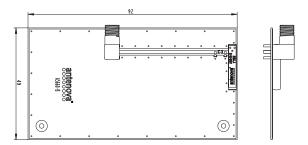
The testboard is designed for evaluation purposes for Mica 2.4 GHz SMD antenna. The board has the same size as a typical PCMCIA card and is fitted with an SMA connector.
